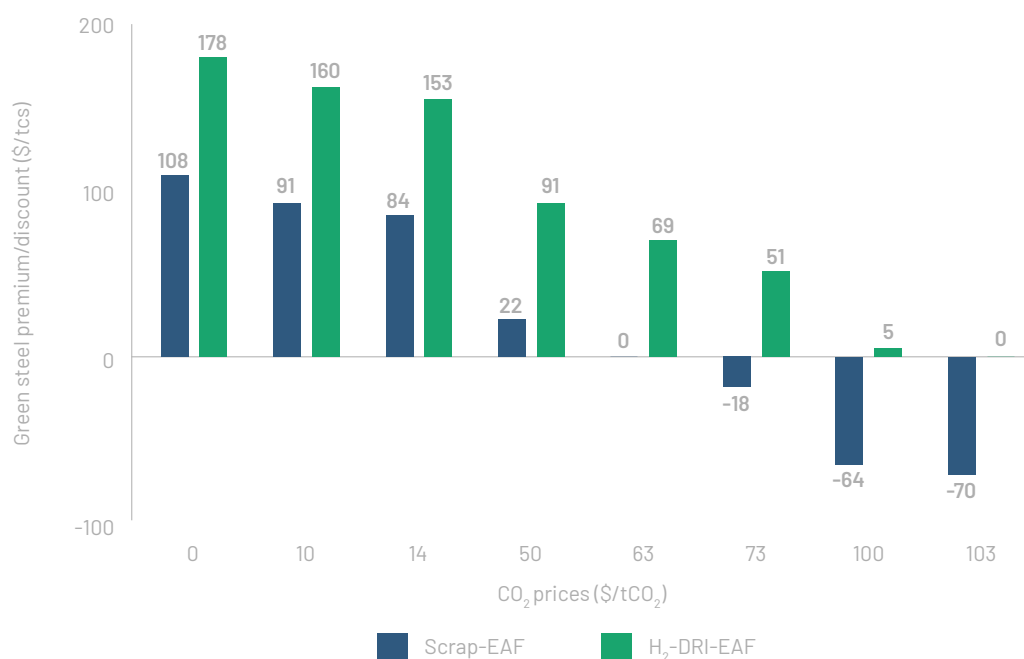
Figure 5: Sensitivity Analysis of CO 2 Prices in Malaysia: Cost Delta of Scrap-EAF and H 2 -DRI-EAF ($/tcs) Compared to BF-BOF Steel at Different Carbon Prices
